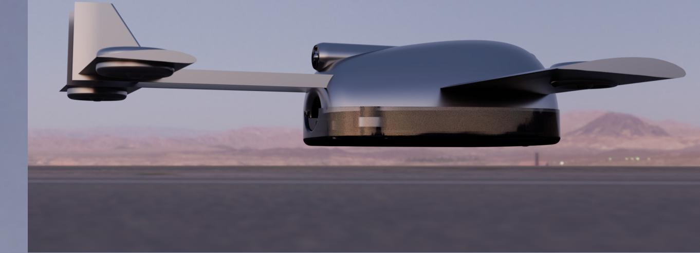
This model is designed for areas prone to wildfires and can house up to 10 extinguishing balls. Drones are stationed at firehouses and autonomously launched when a fire is reported or predicted using our wildfire AI prediction software.
